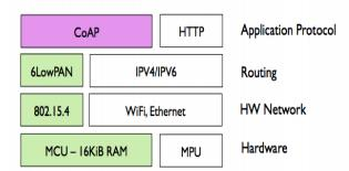
Following the arrival of IPv6, several 'waves' of IoT development can be discerned. First, there was the standardisation work in the lower abstraction layers of the hourglass model. That work included the **6LoWPAN** initiative, for example, which is now being carried forward by the **6Lo** WG. And, in 2015, <u>RFC7668</u> came out, standardising IPv6 over Bluetooth Low Energy (BLE).
