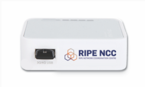
A RIPE Atlas (v3) hardware probe
