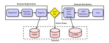
Figure 1: TLD operations: registration (left), domain resolution (right), and datasets.
